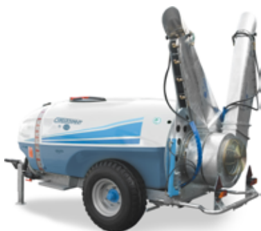
ATC F2D 2 CANNONS GROUP 450 MM with double-suction turbine
