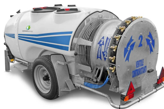
ATD EX 600-800-1000 litres with double axial counter rotating fan for orchards and vineyards
